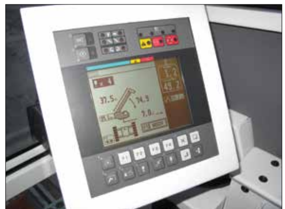
TADANO AML-C rated capacity indicator provides continuous feedback of crane lift position and data.
