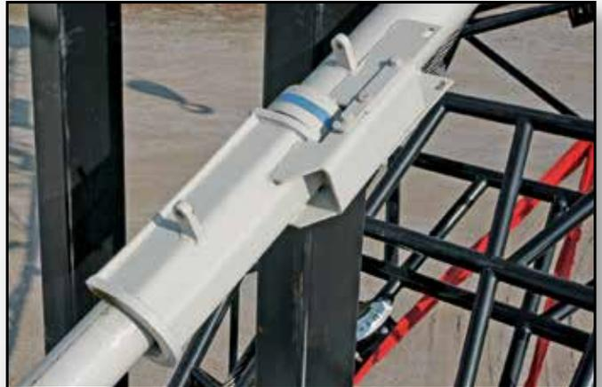
Spring-loaded 90° backstops unpin and rotate, allowing boom to go to 90° for luffing attachment
