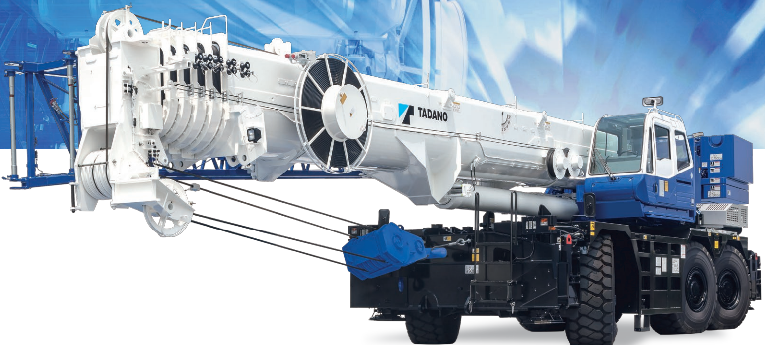
Photo: Hydraulic offset jib
