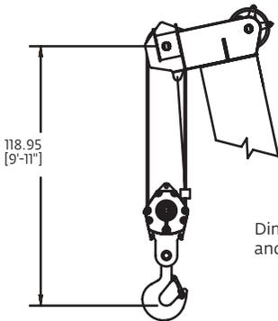
Dimensions are for largest Grove furnished hookblock and overhaul ball, with anti-two block activated.
