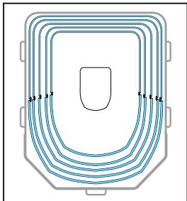
The proven "U" shaped **MEGAFORM™** boom design provides a natural cradling position for boom sections which eliminates stiffeners—thus reducing weight and increasing capacity. Large wear pads provide superior boom alignment when telescoping and allows an excellent transition of weights between sections.
