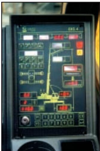
Monitoring the lifting condition of the crane at all times, EKS4 works together with, but independently of the ECOS as a complete command and control system, or separately as a load moment indicator. Continually running fault analysis, the system advises service codes which can be transmitted to any Grove service center, allowing fast accurate investigation and recommendation.
