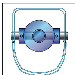
The unique **TWIN-LOCK™** boom pinning system automatically pins the sections in position using two horizontal large diameter pins, which increases security. A single telescope cylinder inside the boom reduces weight which has been used elsewhere to strengthen the machine.
