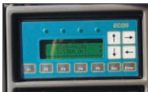
While the operator is concentrating on the lift, ECOS (Electronic Crane Operating System) is busy monitoring and controlling all of the principle crane functions and providing exact telescoping status on its fully graphic in cab display.
