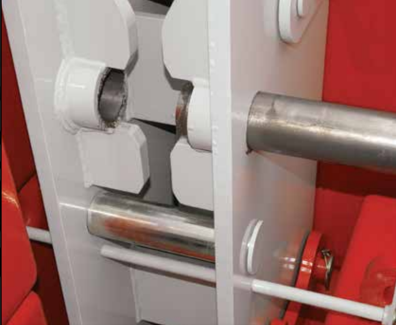
Simple lever action disengages counterweight pins from upper
